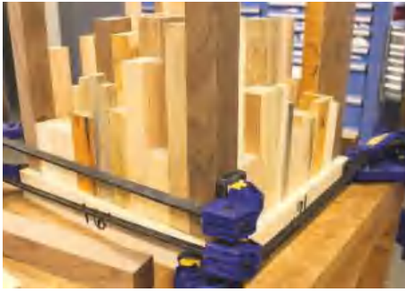
▲ Pic.3 Use clamps to hold everything together, with more pieces of scrap at the sides
